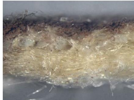
Finest particles in the depth of the needlefelt
